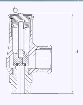
Maximum permissible built up back pressure = 10% of set pressure at or below which flow is not reduced. Stable operation on flows down to 50% of valve rated capacity.
